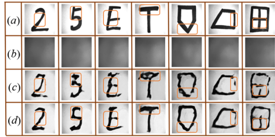
Fig. 5. Visual performance comparison between MPLF and SPLF frameworks on the untrained targets with different structures. (a) Ground truth. (b) Scattering images with polarization directions of 0^\circ . (c) Reconstructed images by SPLF framework. (d) Reconstructed images by MPLF framework.
